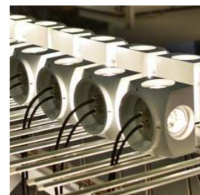
7 Testing of the luminaires
